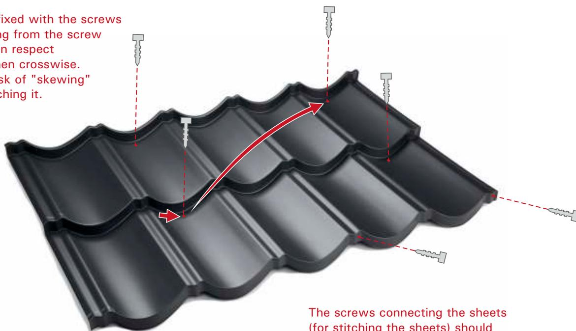
The screws connecting the sheets (for stitching the sheets) should be tightened only after complete fixing of the sheet to the battens.
